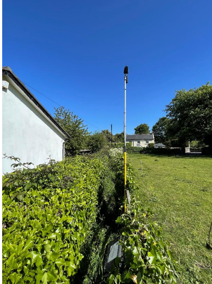
Figure 5: Noise Logger Setup
