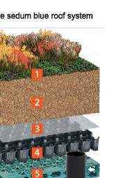
Paving or decking to suit project requirements. Typically 50mm+ Height 0.94 to 18.88 per landscaping surface finish above the deck to create a 17 to 1070 pedestal Waterproofing waterproofing system included ST flow restrictor and overflow 25-1120 Varies Please note: This system should not be used as part of an inverted blue roof system, due to the additional ballast that may be required. Bauder blue roof systems require bespoke flow rate calculations please contact our technical department
